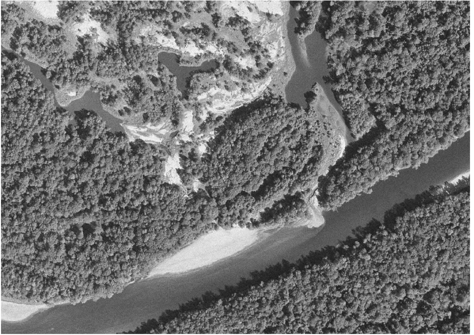
1993: Sand deposition out of sand mine at Big Escambia Creek confluence. Note areas previously with open water are silted in. Very small outfall. Sand washing overland to deposit downstream of old channel.
